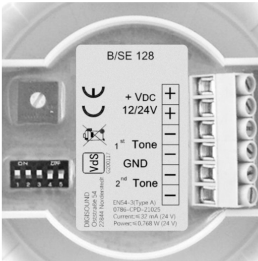
Connector and label inside B/SE 128
